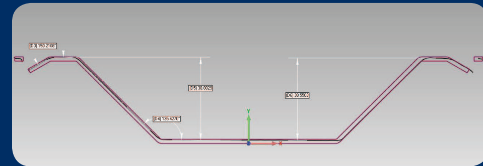
Figure 7: Comparison of scan to 3D CAD model
