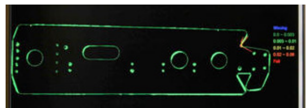
Figure 2: Inspection Report of the 2D component
