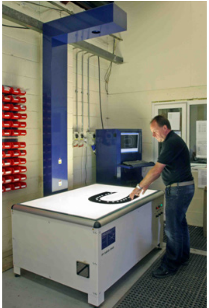
Figure 3: Chris Whitwam inspecting a routed aerospace component on the InspecVision Planar P120.50 measuring machine
