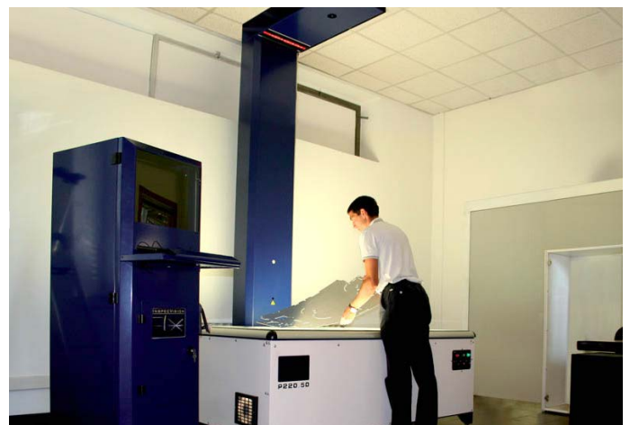
Figure 3: Planar (P220.50) inspecting a sheet metal part at Verona Lamiere
