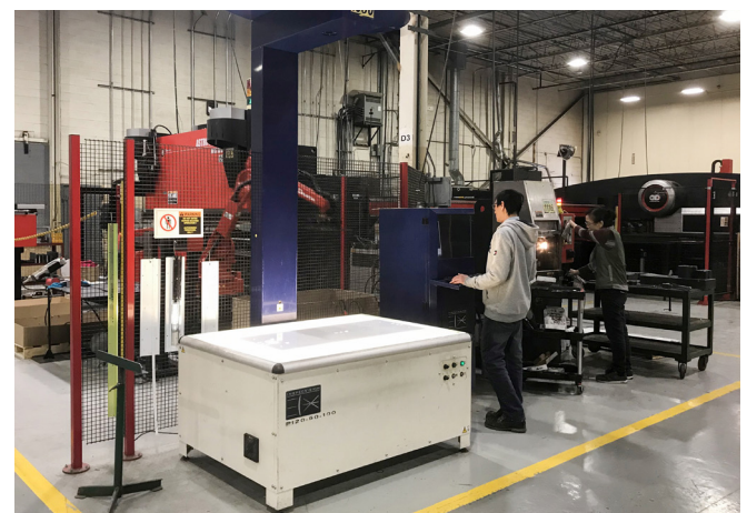
Figure 3: Viscor operator measuring a part on the Planar machine.
