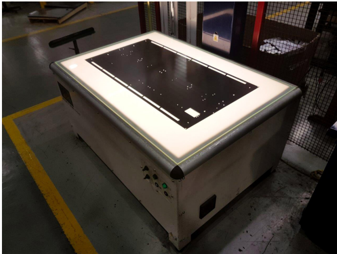
Figure 4: Large part being measured on the Planar P120.50.
