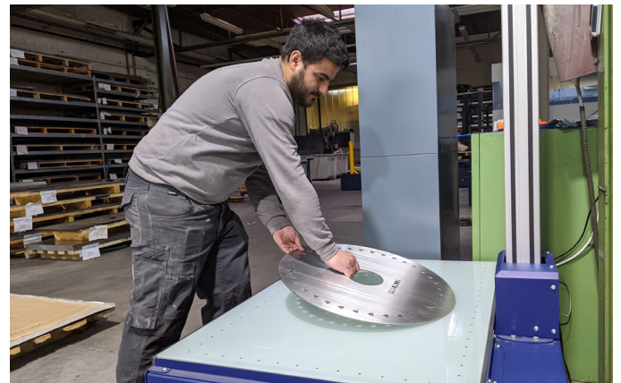
Figure 2: Disc being placed on Planar system for inspection.
